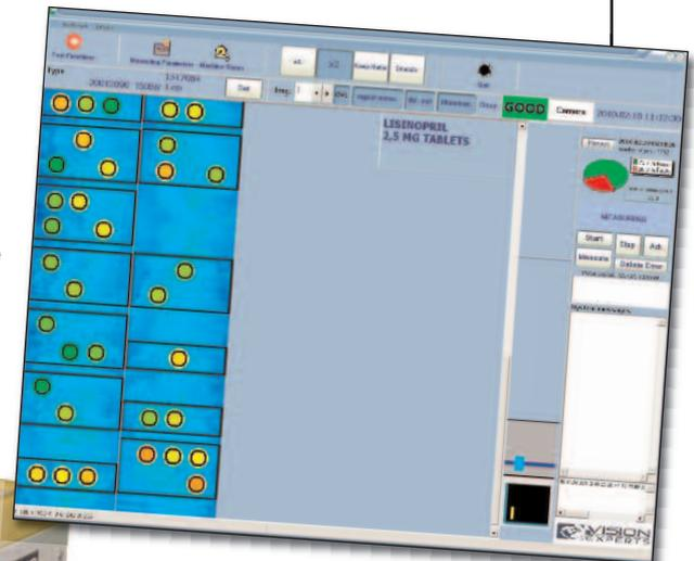
**Left: Vision-Expert's optical inspection machine can measure the exact height of the Braille dots at high-speed. Right: The controlling software is run on a regular industrial PC in Windows settings and has a user-friendly graphical interface. The software can store up to thousands of measuring programs. Below: The series of photographs taken of the laser line draw a three-dimensional "map" of the surface of the carton.**
